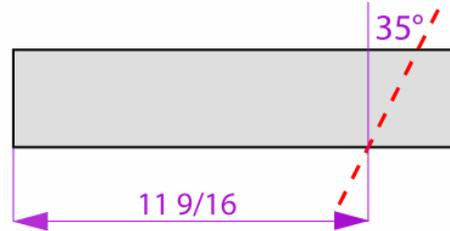
Use a *Leg* segment you've already cut as a guide by flipping it, stacking on top and lining up the mitered edge with the mitered edge of the lumber. Crosscut the lumber at the *Leg* segment butt end. Now cut a **48 in** segment. Then cut an **18 in** segment. This last segment will be the *Cross Beam*. Discard the approximate scrap.
