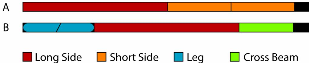
frame. Use these **48 in** and **21 in** segments as templates for making similar cuts. Cut another **21 in** segment. Discard the approximate 6 in scrap.
