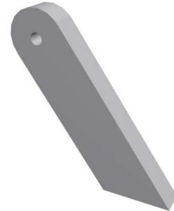
Granted the circular pivots are structurally and aesthetically beneficial, but they do take a certain degree of craftsmanship to achieve. Fortunately, any contour will also work so long as the cut-lines are inside of a bounding radius of 1.75 in. A common alternative to circular legs, are notched ones. One can simply notch the legs by cutting 2 opposing 45° miters and then taking down the point with a cross cut or sanding.
