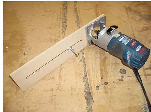
3 inches away from the center mark.) Then set up your jig on the boards, turn on your tool, and rotate around the center mark until you've cut out a circle.
