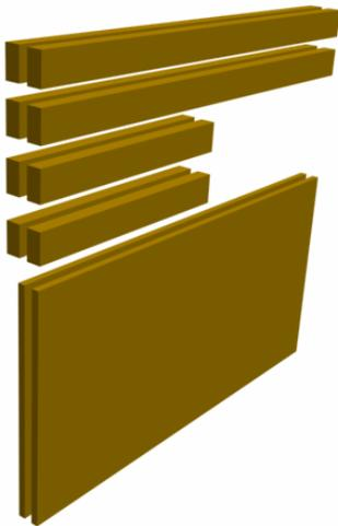
Gather the **48 in** and **21 in** segments and plywood sheets. If framing or box clamps are available to you, now would be a good time to grab them. Mock up or “dry fit” the pieces together on level ground. The longer segments should sandwich the shorter ones between them.
