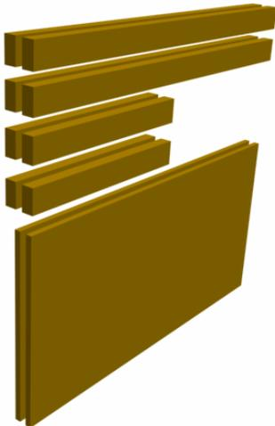
Gather the **48 in** and **21 in** segments and plywood sheets. If framing or box clamps are available to you, now would be a good time to grab them. Mock up or “dry fit” the pieces together on level ground making sure that all the rip-cut sides are facing down. The longer segments should sandwich the shorter ones between them.
