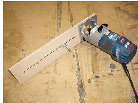
edge of the cutting blade 3 in. Drill a pivot point into the center mark on the board and a starter hole on the circumference of the circle (anywhere 3 inches away from the center mark.) Then set up your jig on the boards, turn on your tool, and rotate around the center mark until you've cut out a circle.
