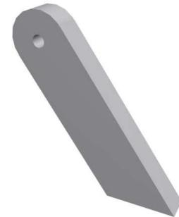
Granted the circular pivots are structurally and aesthetically beneficial, but they do take a certain degree of craftsmanship to achieve. Fortunately, any contour will also work so long as the cut-lines are inside of a bounding radius of 1.5 in. A common alternative to circular legs, are notched ones. One can simply notch the legs by cutting 2 opposing 45° miters and then taking down the point with a cross cut or sanding.
