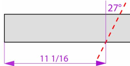
Use a *Leg* segment you've already cut as a guide by flipping it, stacking on top and lining up the mitered edge with the mitered edge of the lumber. Crosscut the lumber at the *Leg* segment butt end. Now cut a **48 in** segment. Then cut an **18 in** segment. This last segment will be the *Cross Beam*. Discard the approximate 6 in scrap.
