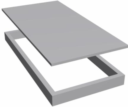
Drill pilots through the plywood into the box frame about every **6 in.** Placement will matter for aesthetic reasons if you are not planning on painting eventually. Also make sure not to drill into the horizontal screws holding the box frame together.
